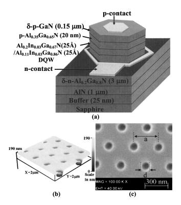
FIG. 1. (a) Schematic diagram of 333 nm UV LED structure showing mesa and contact pads. (b) AFM image of the PCs on UV LED with a=600 nm and d=200 nm. The etch depth is around 190 nm. (c) The SEM image of the PCs on UV LED with lattice constant a=300 nm and hole diameter d=100 nm.
